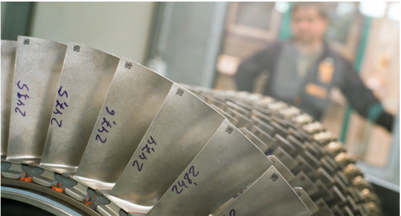
ABOVE: A CFM56 HIGH-PRESSURE COMPRESSOR IN BUILD AND BALANCE. Image courtesy of Lufthansa Technik.
